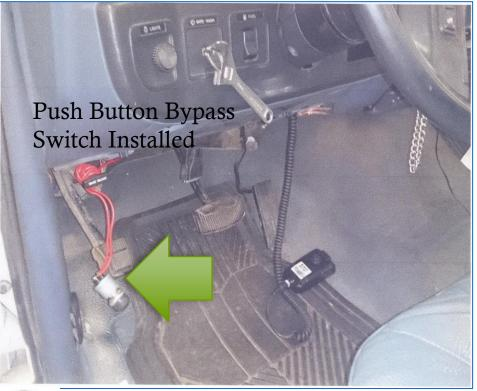
A Bypass Switch interrupted the ground and hot wires prior to reaching the BAIID
